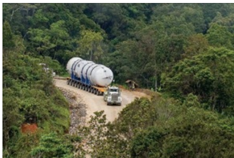
A vessel is transported to the Hides gas plant site through the unique PNG terrain.
