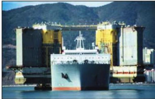
*Towing the hull of the Tension Leg Platform to its location on the Kizomba A development in Angola. It will be set in a water depth of 3,850 feet.*
