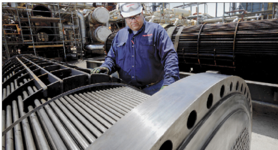
An engineer inspects a modified heat exchanger tube bundle prior to installation at a U.S. Gulf Coast refinery.
