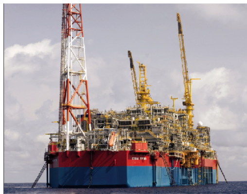
The Erha FPSO has tiebacks to over 30 subsea wells with a capacity of over 200 thousand barrels per day.
