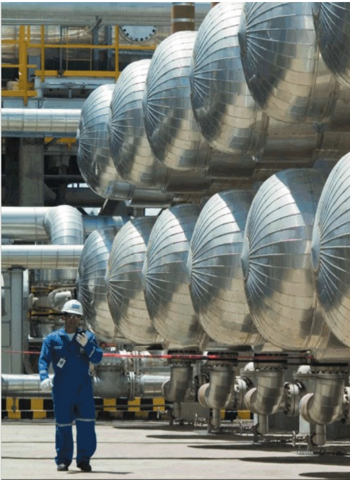
Diluted crude oil is treated at the Cerro Negro central processing facility, Venezuela, to remove associated gas, water, and salt. The crude is then transported approximately 185 miles to the Cerro Negro Upgrader for upgrading to a synthetic crude oil before shipping to the Chalmette refinery in the United States.
