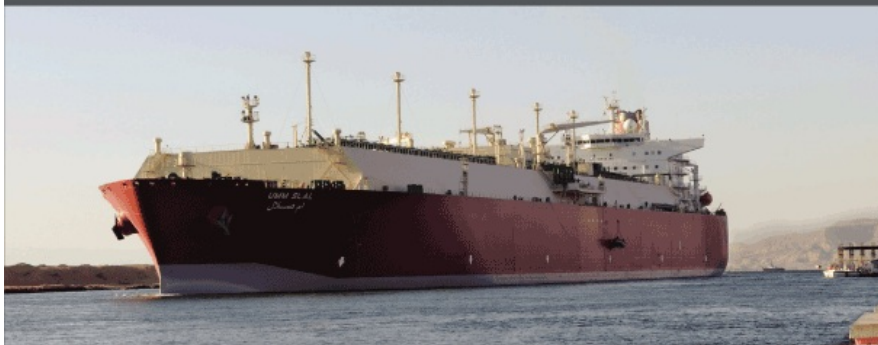
The Q-Max LNG carrier Umm Sial passes through the Suez Canal on its way from Qatar to the United Kingdom. The combination of the world's largest LNG trains and carriers allows gas from ExxonMobil's joint ventures in Qatar to be marketed competitively around the world.
