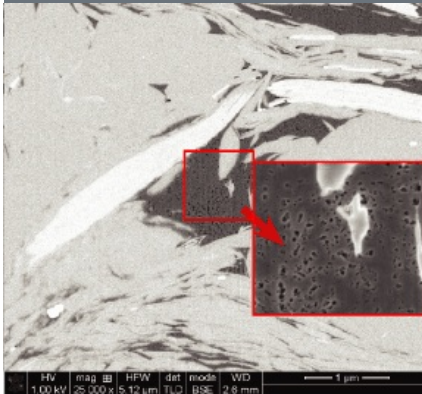
High-resolution electron microscope imaging is used to study the structure of shale gas reservoirs, an increasingly important source of natural gas production. Shale pores can be as small as one-billionth of a meter in size.
