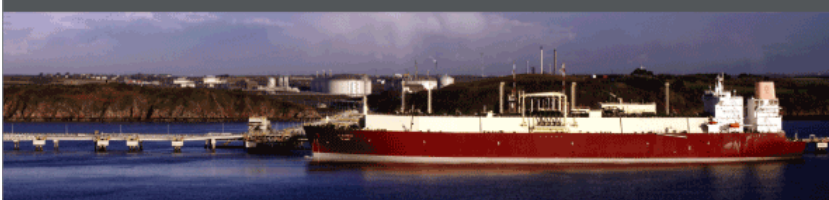
The South Hook LNG regasification terminal opened in 2009 and will have the capacity to deliver 2 billion cubic feet of gas per day. It will be supplied with LNG from Qatar's North Field using the world's largest carriers, including the Q-Max vessel Al Samriya pictured here.
